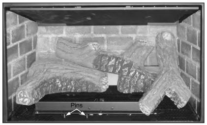
Figure 73: The center of the **right log** fits onto the locator pin on the **back right log** (see Figure 72). The front of the log is to rest on the burner and the back end of the log rests on the back brick panel. Ensure the log does not block any burn ports.
